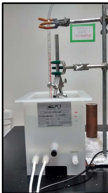
B. 1 MHz reactor
