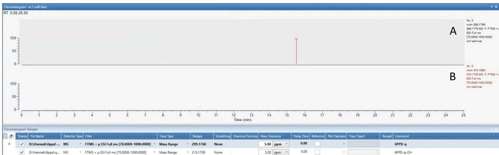
Figure S1: Example chromatograms of negative control RTL-W1 cells for A) parent 6PPD-quinone ( m/z = 299.1760 ) and B) suspected mono-hydroxy metabolite ( m/z = 315.1709 ) identified using a full-scan MS/dd-MS2 method. Full MS extracted ion chromatograms are filtered with 5 ppm mass tolerance. Negative controls were not exposed to 6PPD-quinone, hence the lack of detection.
