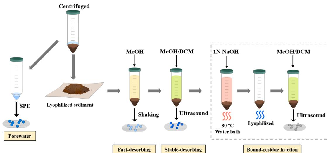
**Fig. 2.** Process diagram of the sequential extraction procedure to obtain rapidly-desorbing, stable desorbing, and bound residue fractions of lyophilized sediments after separation of porewater.
