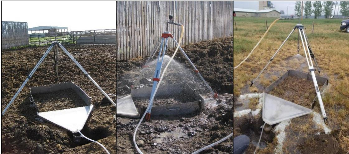
**Figure S1:** Photograph of the Guelph Rainfall Simulator II prior-to (left) and during (middle) a pen-runoff experiment and during a pasture-runoff experiment (right).
