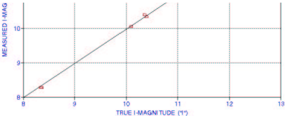
Figure 31. All 13 M67 comparison stars were subjected to the MaxIm DL aperture photometry using a set of 8 I-filter images (using the "8E/Schuler" system) and the system solution for I-magnitudes is plotted versus "true" I magnitudes. The RMS differences with respect to the 1:1 line is 0.042 magnitudes.
