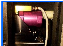
detailed view of the cross-dispersing prism train within its mount; the whole train can be rotated manually (when aligning the spectrograph) with the Newport stage included in its base;
