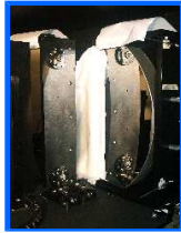
detailed view of the 204mm wide and 408mm long R2 diffraction grating in its mount (inspired from the feros design); the grating is tilted downwards (with 6 invar pins glued on its rear and side surfaces to hold it against gravity) to minimise dust accumulation on the diffracting surface, and semi circular baffles are included in the bottom part of the mount to reduce straylight from the grating to a minimum;
