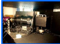
global view of the last section of the spectrograph optics; photons reflected off the transfer collimator (not visible here) are cross-dispersed by the prism train (in its black parallelepipedic cage with two handles on top, on the right of the image) and concentrated by the large dioptric camera (black cylinder with a hook on top of it, in the middle of the image) before being collected onto the ccd detector inside its dewar and vacuum vessel (pink cylinder on the left of the image); the thin disc between the prism train and the dioptric camera is the motorised hartmann mask, used to focus automatically the spectrograph;
