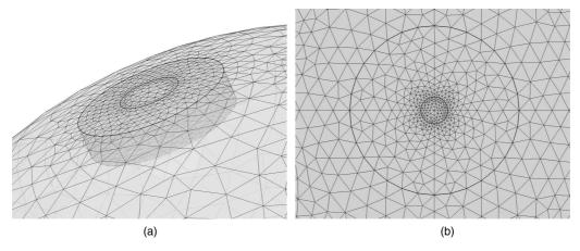
FIG. 2. Illustration of extremely fine and fine mesh regions.
