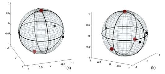
FIG. 16. (Color online) Minimal energy spherical trap configurations for 2N traps of two kinds: (a) 2N = 4; (b) 2N = 6. The radius ratio of the traps is  $\alpha = 10$ . Larger traps are shown in red and smaller in black.
