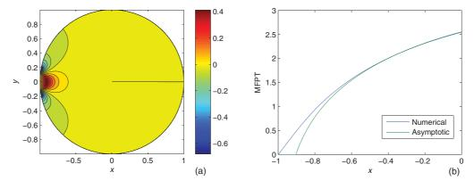
FIG. 13. (Color online) Comparison of asymptotic and numerical results for the MFPT v(x), for a unit disk with one trap of arclength  $2\varepsilon = 0.4$ . (a) Plot of  $v_{num}(x) - v_{as}(x)$  in the disk. (b) Comparison near the trap, along the radius  $x \le 0$ , y = 0.
