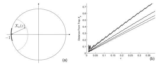
FIG. 14. (a) Relative error measure  $X_a(\varepsilon)$ . (b) Plots of  $X_a(\varepsilon)$  for a = 0.05, 0.1, 0.15, and 0.2 (top to bottom). (Numerical computations were performed for the step  $\delta \varepsilon = 0.001$  in  $\varepsilon$ . Observed oscillations are a numerical phenomenon, which vanishes as  $\delta \varepsilon \rightarrow 0$ .)
