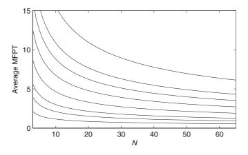
FIG. 19. Trap fragmentation effects. The average spherical MFPT  $\bar{v}$  (2.22) vs N (number of traps) for a fixed trap surface area percentage. Curves for f = 0.1%, 0.2%, 0.3%, 0.5%, 1%, 2.2%, 4%, and 10% (top to bottom).
