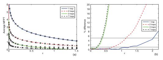
FIG. 6. (Color online) (a) Dependence of the average MFPT  $\bar{v}$  on the trap length  $\varepsilon$  for one-, two-, three-, and seven-trap configurations in a unit disk. The curves correspond to the asymptotic formulas and the crosses to numerical results. (b) Percent difference between asymptotic and numerical results vs  $\varepsilon$ .
