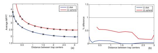
FIG. 12. (Color online) (a) Effect of trap separation in the unit disk (i) and the unit sphere (ii). Comparison of asymptotic and numerical results for the MFPT  $\bar{v}$ . Unit disk: two traps of arclength  $\varepsilon = 0.05$ . Unit sphere: two circular traps of radius  $\varepsilon = 0.2$  located on the equator. (b) Percent difference between the asymptotic and numerical results.
