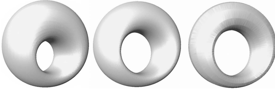
Fig. 1. Three toroidal magnetic surfaces of an anisotropic flux tube configuration. These surfaces are nested one inside another from the right to the left. They are displayed separately for clear visibility purposes.
